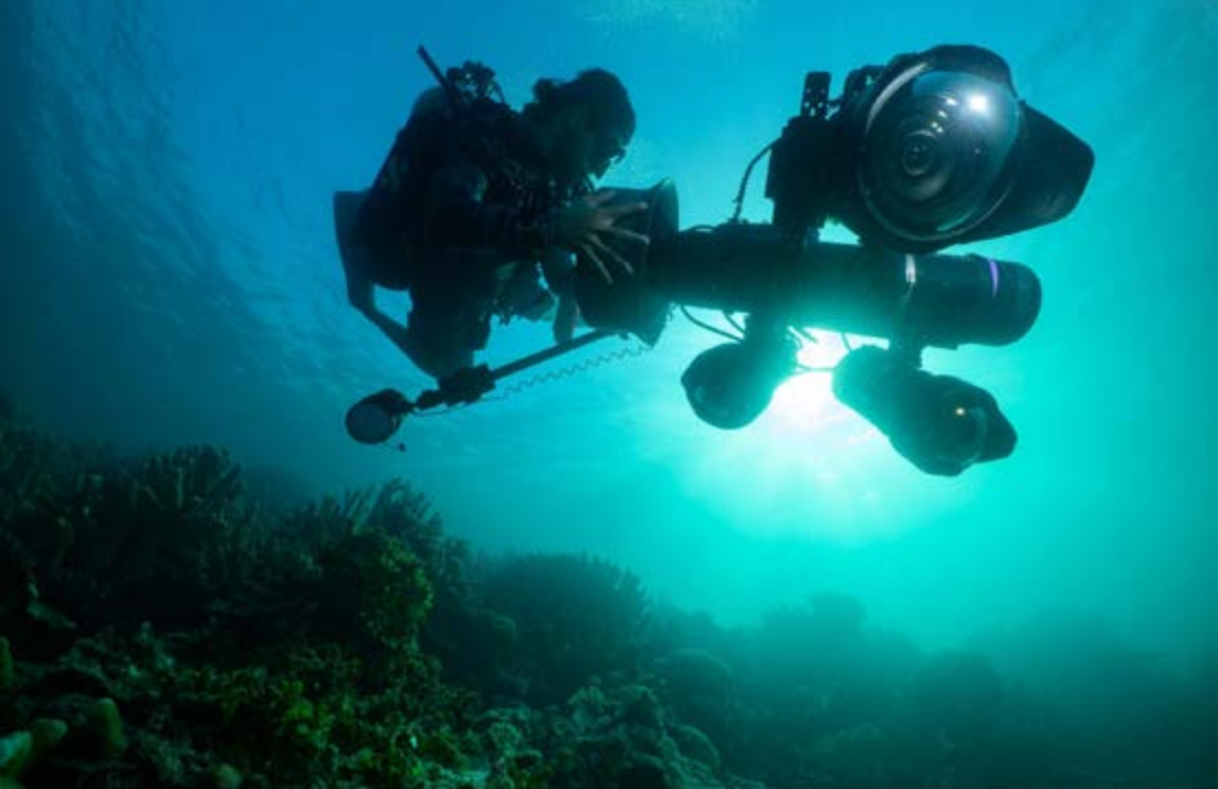
Figure 6. The scooter-based three-camera optical array, designed in partnership with Wild Technologies, was used for rapid imaging across underwater transects (image credit: Jason Gulley).
