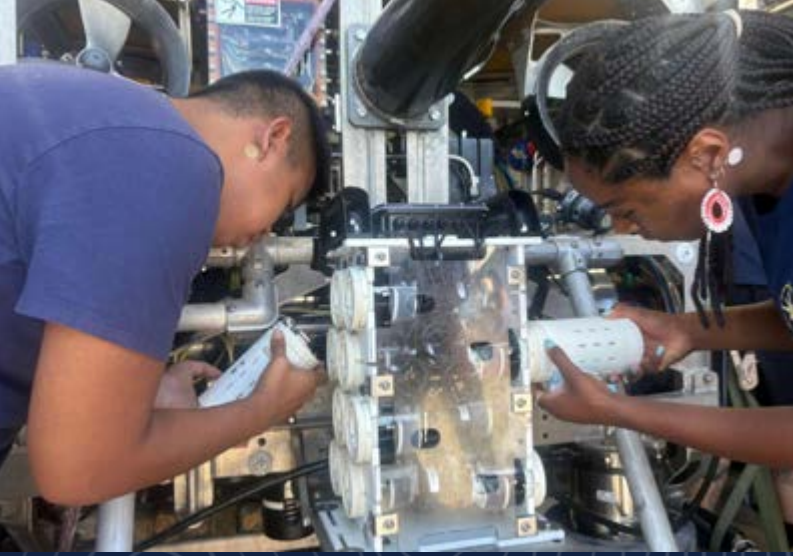
Figure 2. Mounting eDNA filter cartridges onto the MultiPuffer eDNA sampler (image credit: Annette Govindarajan, Woods Hole Oceanographic Institution).
