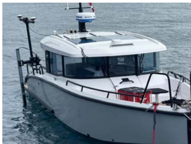
Figure 7. M/V Berry Ferry in survey configuration with the pole and multibeam deployed (image credit: Kristopher Kransosky, Seaward Science).
