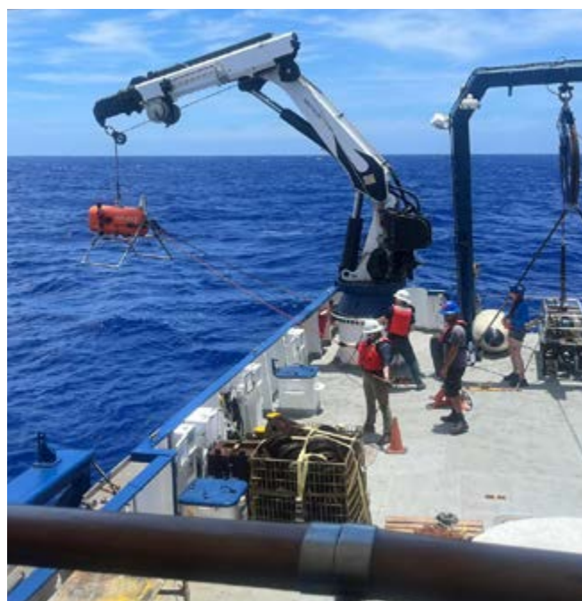
Figure 2. The Orpheus AUV being launched over the side of E/V Nautilus for a dive to a depth of 5,700 meters.
