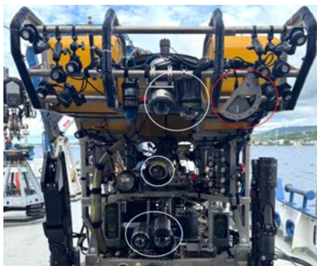
Figure 1. The front of ROV Hercules showing its many cameras, video lights, and sensors. Its high-resolution imaging systems are highlighted with white circles and the Norbit multibeam sonar is shown with a red circle.
