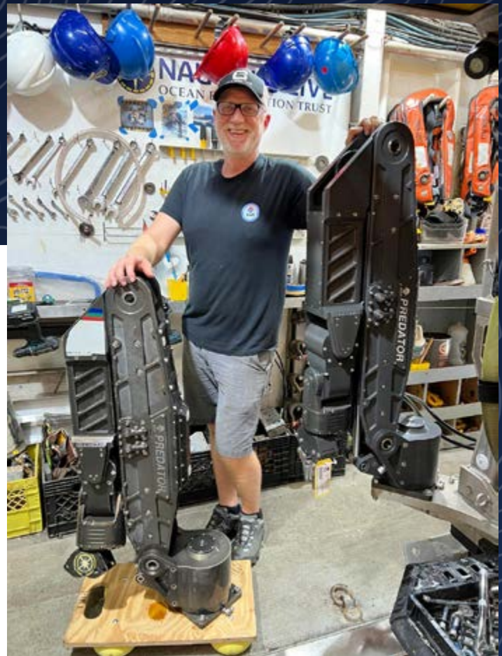
Figure 1. A passing of the torch for ROV Hercules . The legacy Kraft manipulator arm (left), which had been in continuous service since ROV Hercules was commissioned in 2002, is shown alongside its newly installed replacement (right). Over more than two decades of operations, the original arm supported thousands of scientific sample collections and seafloor interactions. After more than 20 years of dependable service, it has been retired, making way for a new Kraft arm that will continue supporting deep-sea science for years to come.
