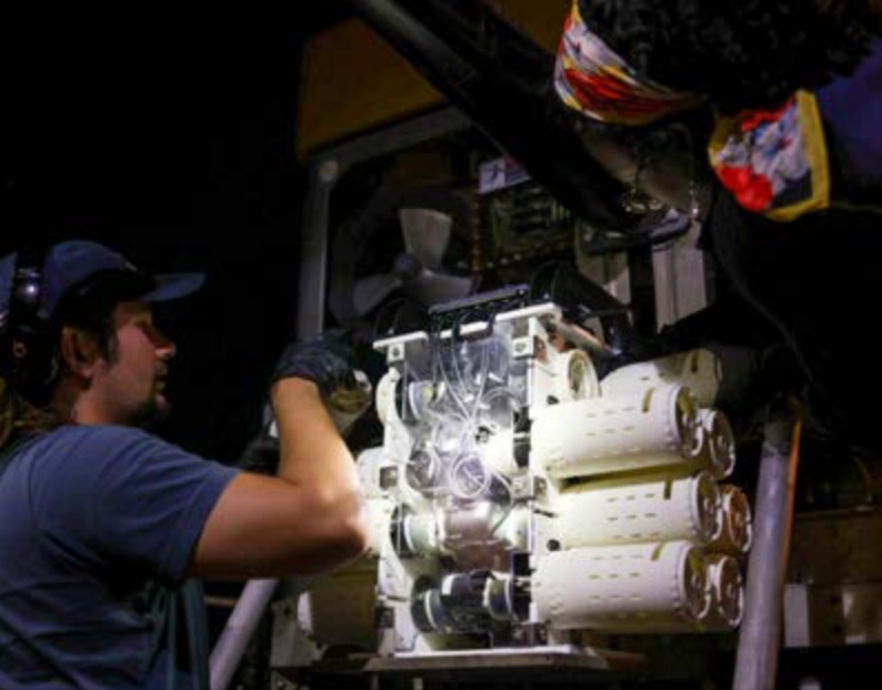
Figure 4. During operations in the Marshall Islands, the Aquatic Labs MultiPuffer autonomous eDNA sampler was integrated onto ROV Hercules enabling the collection of environmental DNA samples alongside seafloor mapping and ROV surveys.
