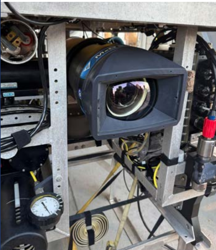
Figure 2. The UHD MXD camera mounted on ROV Little Hercules during integration ahead of the 2025 Cook Islands expedition. This close-up photo captures the first deployment of the system on ROV Little Hercules —and its first journey to abyssal depths—marking a milestone for both the camera and the vehicle as they ventured deeper than ever before.
