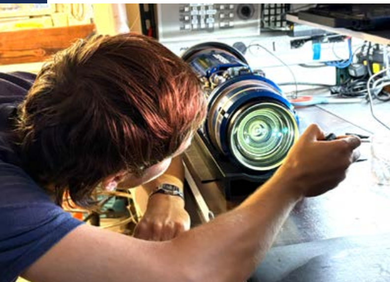
Figure 3. DeepSea Technology Specialist Mikhail Rossoshanskiy inspecting the corrector lens cell in the onboard ROV shop before reassembling the MxD SeaCam (image credit: Aaron Steiner, DeepSea).
