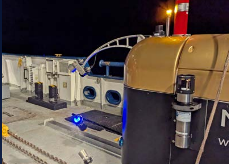
Figure 4. An optical lure was added to Mesobot prior to the NA164 expedition. Similar to the lures on anglerfish, Mesobot 's lure uses lights mounted on the front of the vehicle to attract animals near its cameras.
