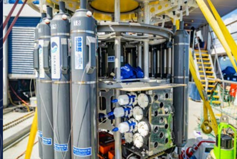
Figure 1. For the 2024 season the team integrated a large-volume eDNA sampler onto the Deep Autonomous Profiler , which enabled the collection of filtered eDNA samples at pre-programmed depths.
