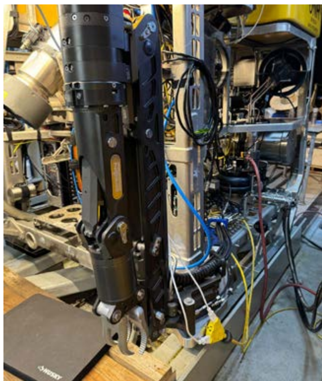
Figure 3. The ROV team installed a new Schilling Orion 7RE manipulator arm on ROV Hercules , which offers superior functionality, reliability, and ease of maintenance in comparison to the previous ISE Magnum manipulator arm.
