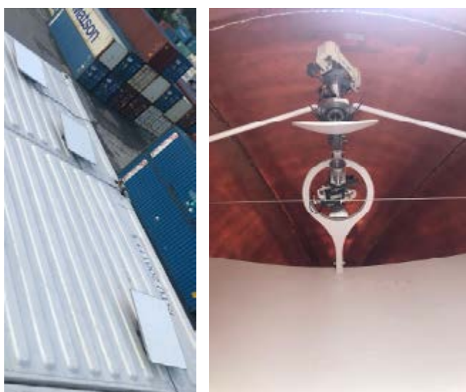
Figure 2. Photographs showing the differences in the onboard antennas required to transmit video streams via Starlink (left) and VSAT (right).
