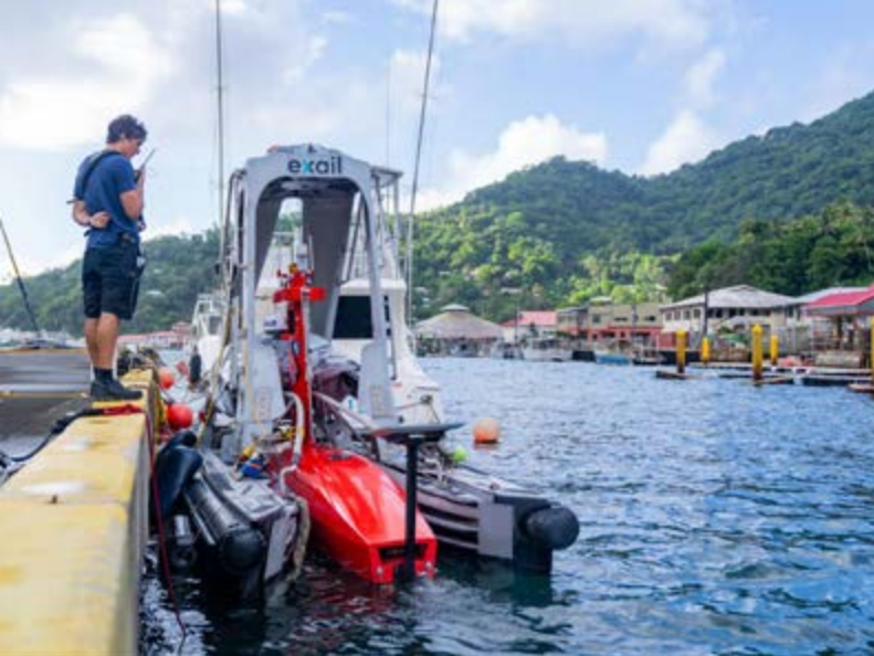
Figure 2. The NA164 expedition to American Samoa used uncrewed surface vehicle DriX launched from a shore-based station in Pago Pago (left), in combination with autonomous underwater vehicle Mesobot and Deep Autonomous Profiler launched from E/V Nautilus (right), to conduct one of the most comprehensive surveys of midwater habitats in American Samoa to date.
