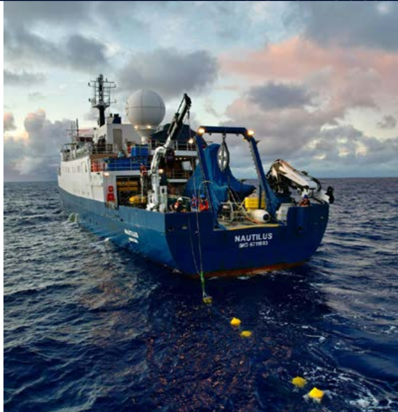
Figure 4. On the last day of the NA163 expedition, the team successfully deployed an acoustic mooring east of Tutuila Island to support cetacean monitoring efforts by the NOAA Cetacean Research Program.
