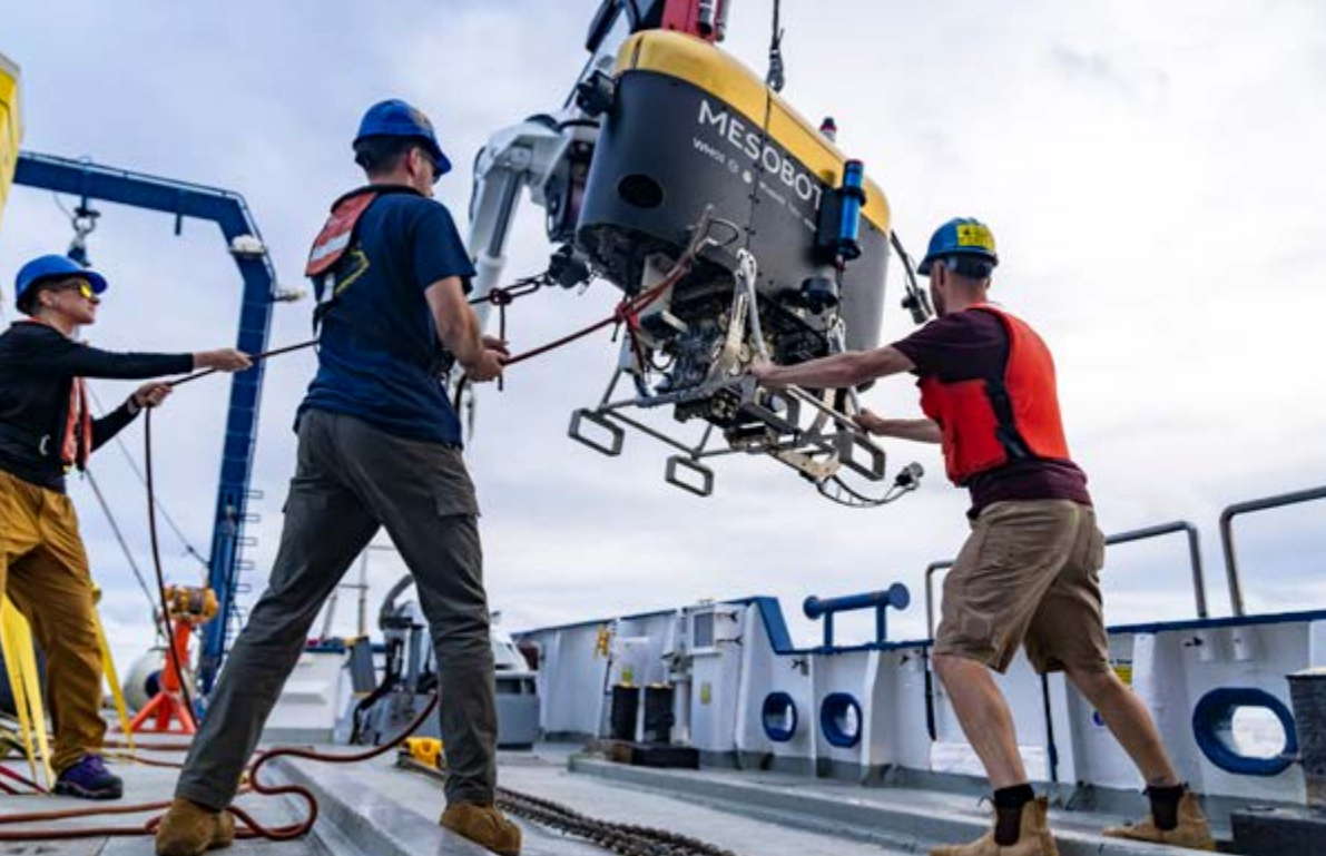
Figure 2. Mesobot being recovered back on deck of E/V Nautilus after a successful dive to explore midwater environments above Vailulu'u Seamount.
