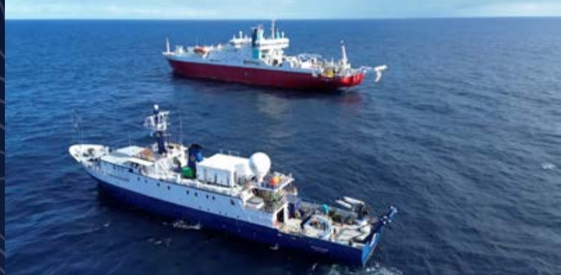
Figure 7. C/S Cable Innovator next to the E/V Nautilus during dual-ship operations to lay a secondary replacement cable at Cascadia Basin.
