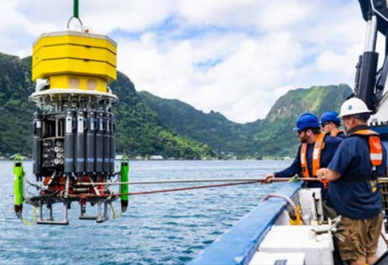
Figure 1. For the 2024 season the team integrated a large-volume eDNA sampler onto the Deep Autonomous Profiler , which enabled the collection of filtered eDNA samples at pre-programmed depths.
