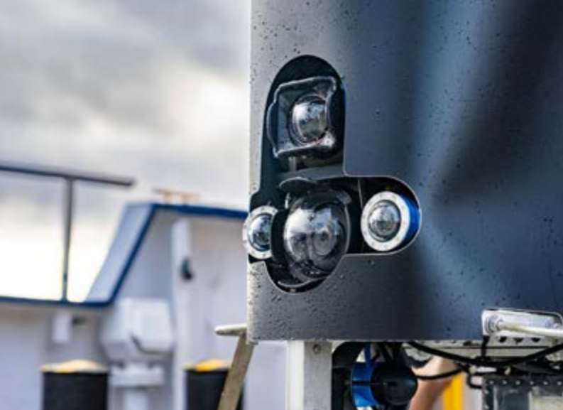
Figure 3. Several upgrades to the imaging systems of Mesobot were implemented prior to the NA164 expedition, including moving the lights out on booms to better shape the light patterns in front of its two cameras.
