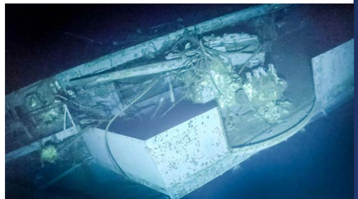
Figure 6. Large cut-outs on the side of USS Yorktown made by its crew in an attempt to jettison the anti-aircraft guns and right the vessel as it listed.
