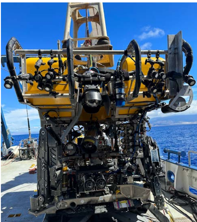
Figure 2. The new Widefield Camera Array installed on ROV Hercules . The system consists of three modular cameras, two that are mounted side by side in the center of the vehicle and a third that is mounted on the upper bumper bar centered amongst the LED lights.
