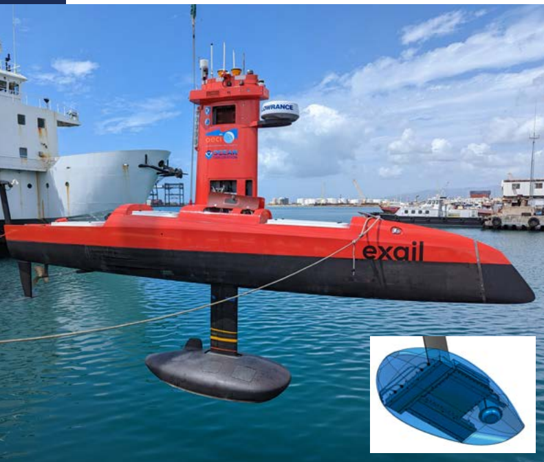
Figure 1. New gondola installed on DriX along with StarLink antenna on small black mast at the aft end of the vehicle. Sketch of new DriX gondola with EM712 (inset).
