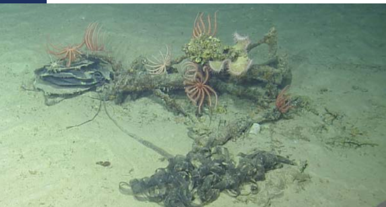
Figure 3. Support strut and delaminated wheel of the Havoc nose landing gear, which was located 63 meters away from the main wreckage.
