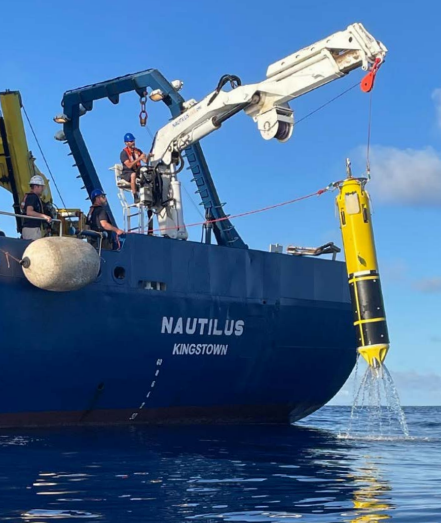
Figure 2. The E/V Nautilus recovering the Hadal Water Column Profiler after a cast during the 2023 shakedown expedition (NA147).
