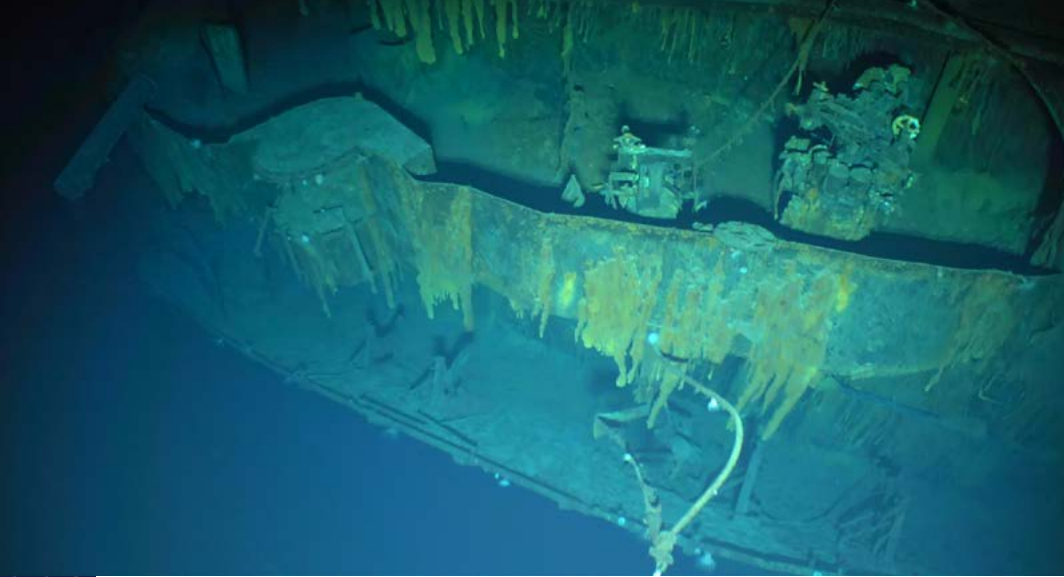
Figure 2. Guntub on the wreck of the Imperial Japanese Navy ship Akagi covered by rusticles, a rust formation produced by deep-water bacteria that oxidize iron and steel.
