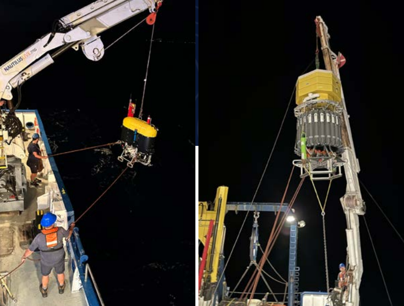
Figure 2. The E/V Nautilus deck team recovering Mesobot after a successful deployment that collected eDNA samples (left). The eDNA samplers are located in the payload area at the base of the vehicle.
