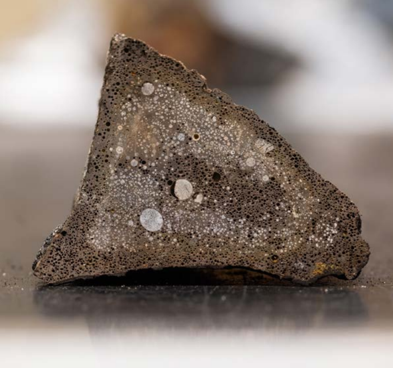
Figure 3. Cut surface of sample NA154-073-C-GSO, showing the gas bubbles from the lava, including a zone where the bubble cavities are now filled with calcium carbonate (light) (photo credit: Sandra Slead).
