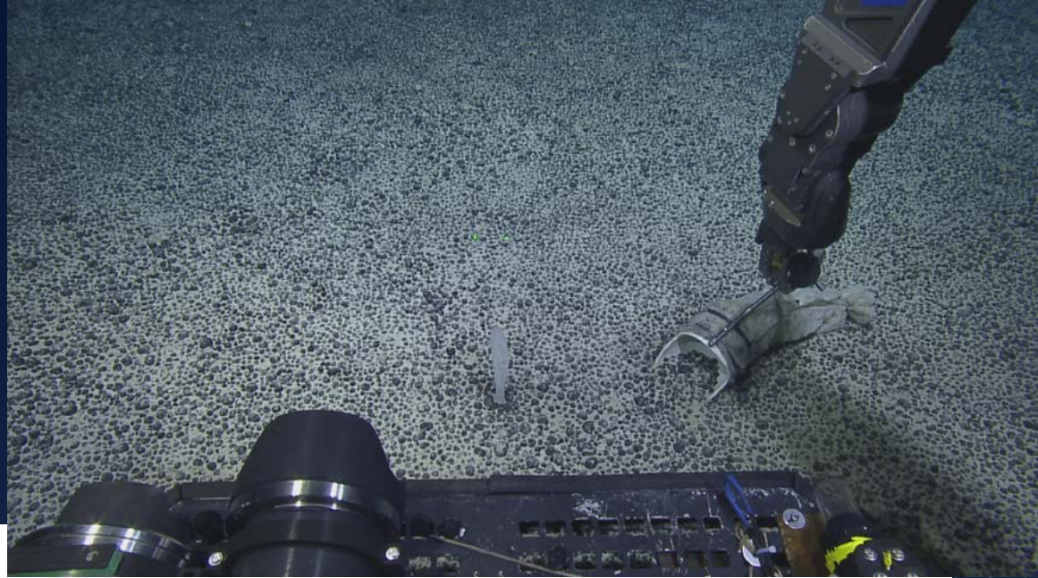
Figure 2. ROV Hercules scooping polymetallic “nuggets” from an expansive flat-lying region south of an unnamed seamount (H1998). Green laser dots mid-frame indicate 10 cm scale.
