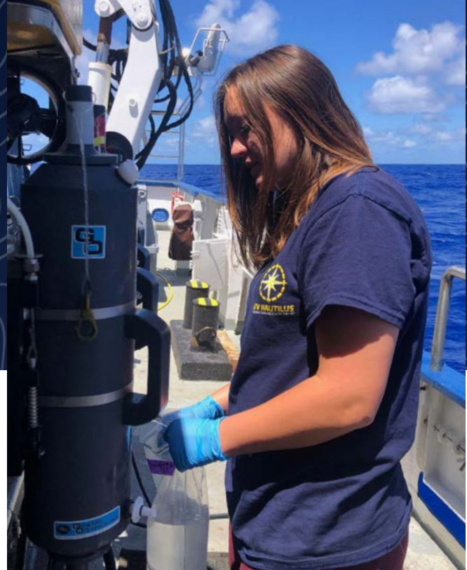
Figure 2. University of Rhode Island graduate student Jane Carrick retrieving an eDNA water sample from the Niskin bottle mounted on ROV Hercules (photo credit: Steve Auscavitch).
