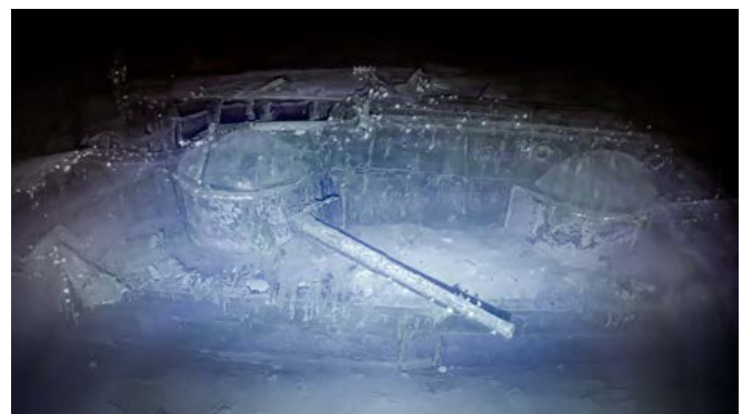
Figure 3. The sides of the Kaga wreck contain 8-inch casemate guns, which were part of the ship-to-ship armament of the vessel's original battleship design before it was converted into an aircraft carrier.
