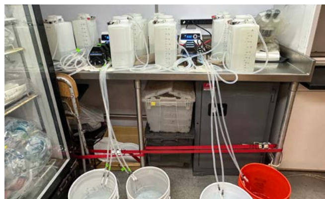
Figure 4. In the E/V Nautilus wet lab, we filtered seawater from the Deep Autonomous Profiler to collect eDNA samples.
