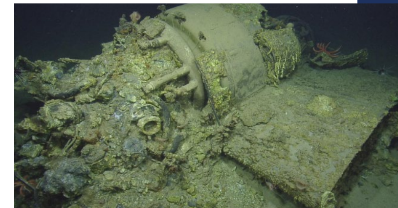
Figure 4. Inverted left wing portion, engine nacelle, and heavily deteriorated radial engine, which was located 79 meters away from the main wreckage.
