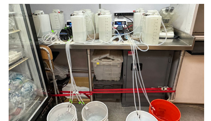
Figure 4. In the E/V Nautilus wet lab, we filtered seawater from the Deep Autonomous Profiler to collect eDNA samples.
