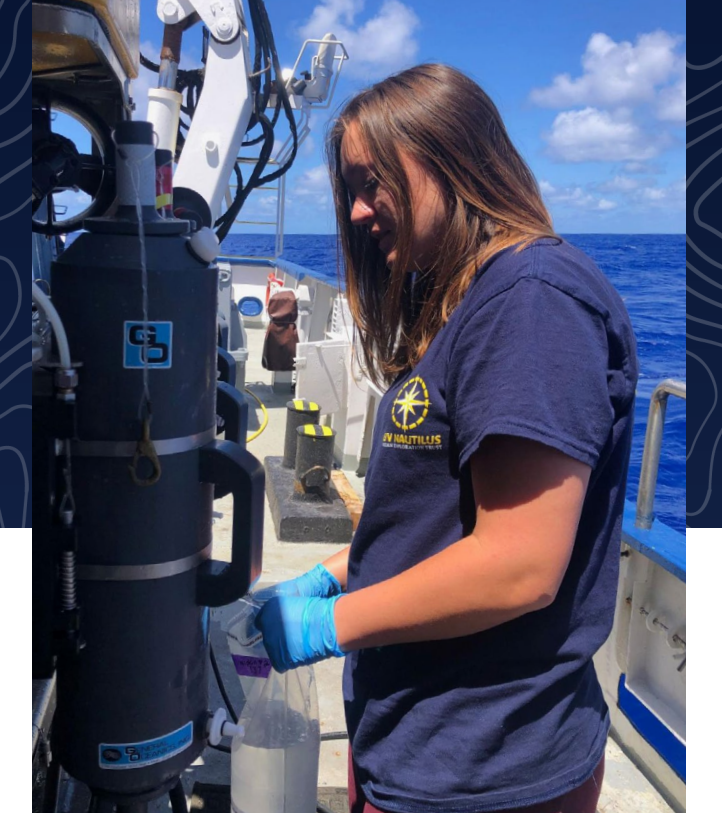
Figure 2. University of Rhode Island graduate student Jane Carrick retrieving an eDNA water sample from the Niskin bottle mounted on ROV Hercules (photo credit: Steve Auscavitch).
