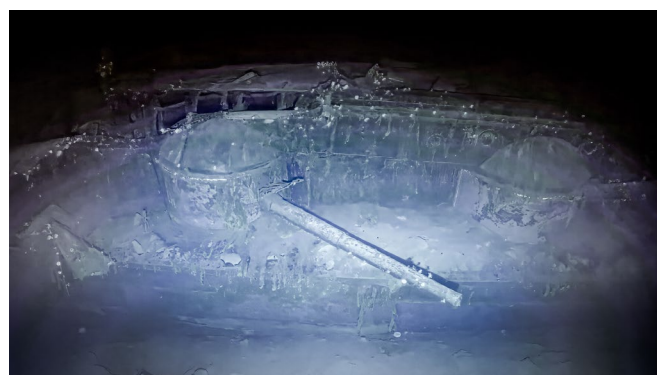
Figure 3. The sides of the Kaga wreck contain 8-inch casemate guns, which were part of the ship-to-ship armament of the vessel's original battleship design before it was converted into an aircraft carrier.
