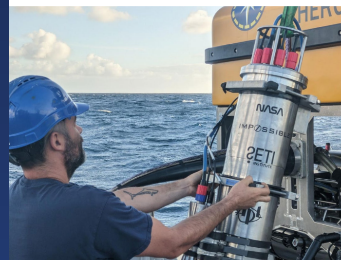
Figure 1. The Laser Divebot being integrated onto ROV Hercules prior to the E/V Nautilus expedition to Kingman Reef and Palmyra Atoll (NA149).
