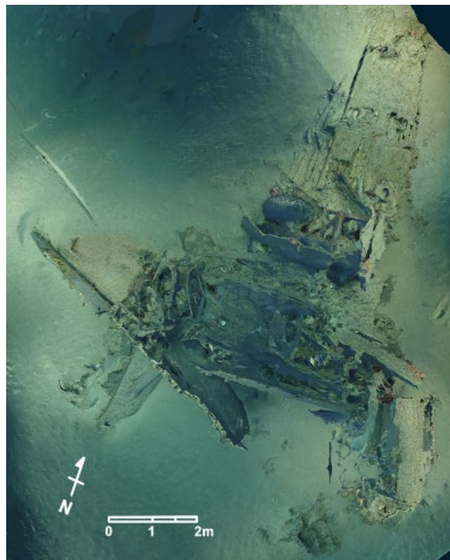
Figure 1. Mosaic of the main wreckage of the A-20 Havoc bomber, which consists of the inverted right wing with landing gear (top), tail empennage (left), and cockpit (lower right).
