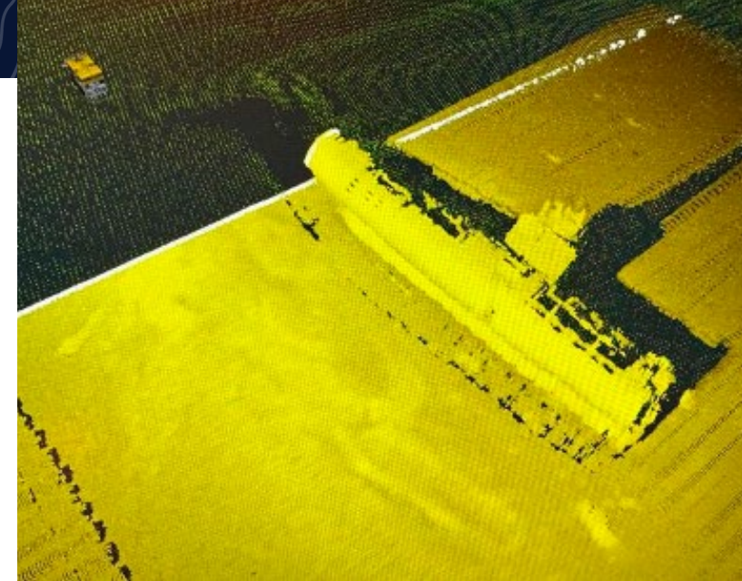
Figure 9. The 14-day Ocean Exploration through Advanced Imaging expedition focused on integrating a new widefield camera and wideband multibeam sonar onto ROV Hercules to build ultra-high resolution models of the seafloor, including two Japanese submarines from World War II scuttled off O'ahu.
