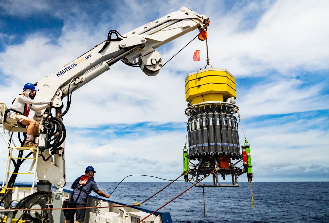
Figure 2. The Deep Autonomous Profiler (DAP) being deployed from E/V Nautilus during the NA157 expedition.
