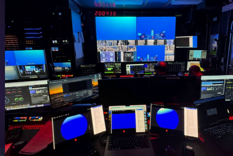
Figure 2. The Widefield Camera Array operated in the control room of E/V Nautilus (left). Stereo cameras and the high-resolution camera mounted on the ROV operate in sync to acquire immersive imaging (right).
