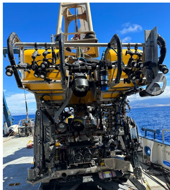
Figure 2. The new Widefield Camera Array installed on ROV Hercules . The system consists of three modular cameras, two that are mounted side by side in the center of the vehicle and a third that is mounted on the upper bumper bar centered amongst the LED lights.
