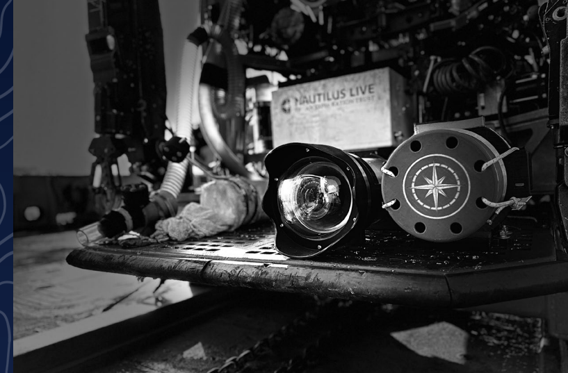
Figure 2. The Widefield Camera Array operated in the control room of E/V Nautilus (left). Stereo cameras and the high-resolution camera mounted on the ROV operate in sync to acquire immersive imaging (right).
