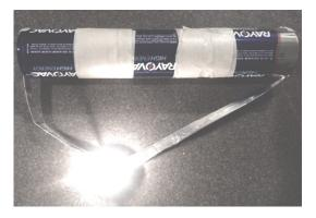
✓ This series circuit was created with insulated wires (remove insulation from ends with wire strippers), masking tape, 1 (9v) battery and 2 (4.5 v) bulbs. Students will notice that based on the voltage of the battery and bulbs they may appear dimmer if they are connected to a lower voltage battery.
