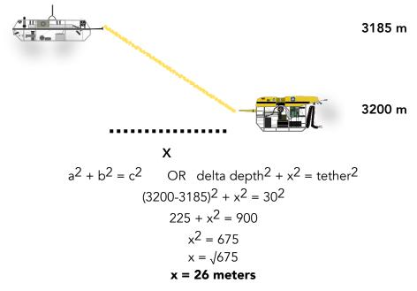
2. If Argus and Hercules are connected with a 50 meter tether, solve for the horizontal range indicated by x.
