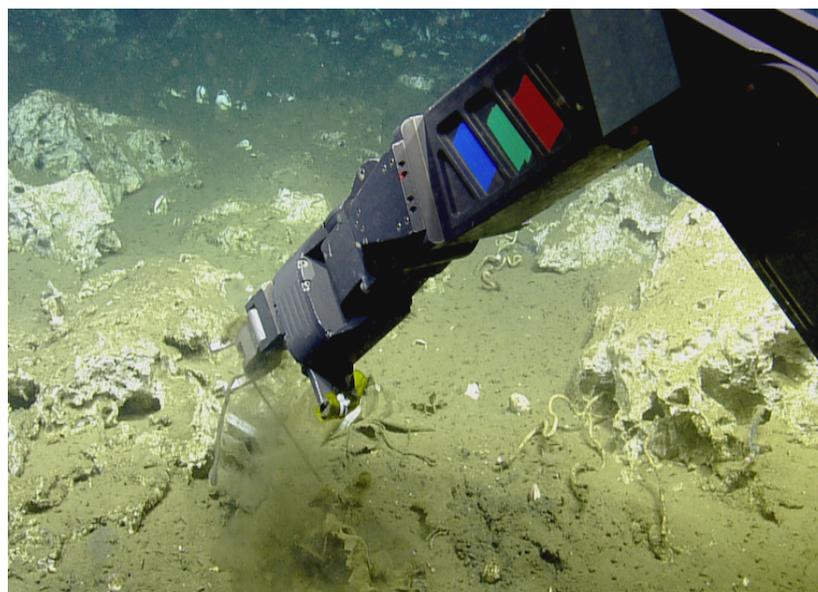
ROV - Remotely Operated Vehicle- *Hercules* had its manipulator arm hooked by discarded line at 1,025 meters off the coast of Southern California. Entanglement hazards like this are a top concern for ROV pilots.
