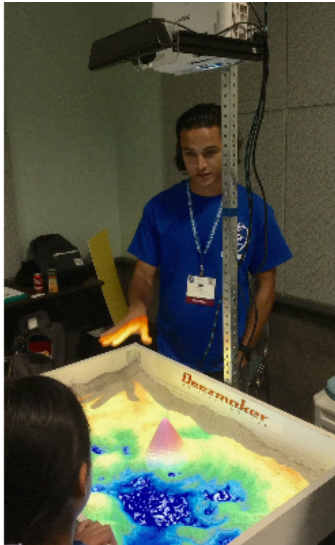
USC Young Scientists Program Intern Bob Steenhuis teaches high school students using the model in Los Angeles. Deezmakers AR Sandbox built with a Xbox-360™ Kinect and projector. Photo courtesy of Dieuwertje Kast.
